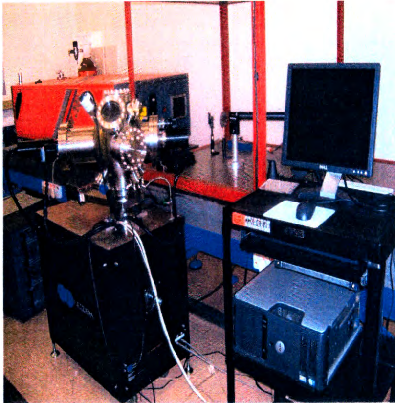
Figure 3.10: 248 nm KrF Lambda Physik excimer laser with PLD setup
